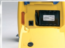
Field replaceable battery
